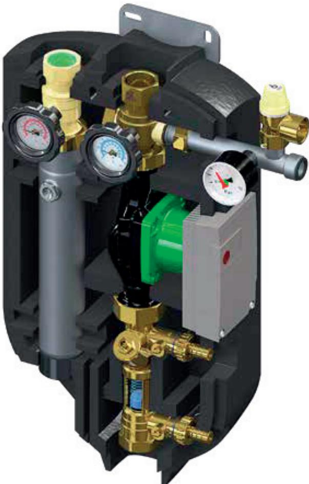
**PORTATA MAX. 2400 l/h****DEBIT MAX. 2400 l/h****SUPERFICIE SOLARE MAX.****80 m<sup>2</sup> (COLLETTORE PIANO)****50 m<sup>2</sup> (COLLETTORE SOTTO VUOTO)****SUPERFICIE SOLAIRE MAX.****80 m<sup>2</sup> (COLLECTEUR PLAT)****50 m<sup>2</sup> (COLLECTEUR SOUS VIDE)**
